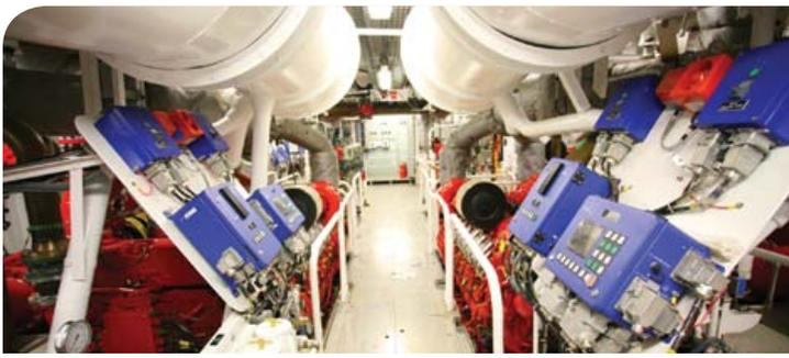
In the engine room of the *Three Forty Three*, four MTU 12V4000 M70 diesel engines deliver propulsion and pumping. The Callosum ship automation system (blue boxes) controls the entire propulsion system and displays the information on one of four touch screens throughout the vessel.
