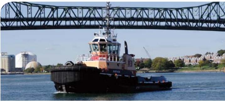
The 30-meter *Justice* was designed to assist LNG tankers and other ships coming into Boston Harbor. Its missions include emergency towing, firefighting and personnel rescue.
