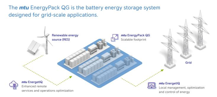
A complete plant design will consist of multiple base units, like the two different variants on the left. Each base unit is designed for 3.7 - 8.8 MVA nominal charge and discharge power, and up to 32.6 MWh nominal capacity. Each battery rack or container has integrated control, fire suppresion and liquid cooling
