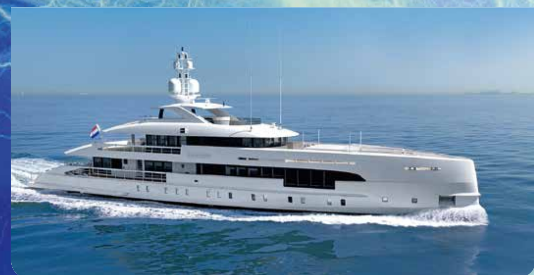
Built by the Dutch Heesen yard, the yacht 'Home' has two 1,200 kW MTU diesel engines and two 110 kW electric motors on board.
