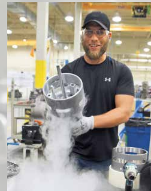
The operative immerses a bearing bushing in a vessel filled with liquid nitrogen with the aid of a jig. The bearing bushing contracts when chilled...
