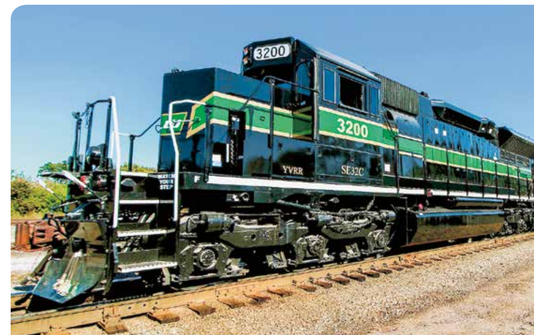
Tier 4-certified locomotives from US manufacturer Knoxville Locomotive Works are powered by MTU Series 2000 and 4000 engines.
