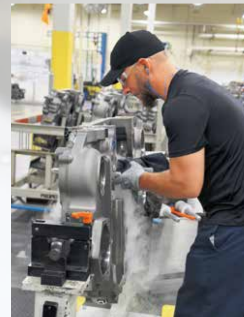
...and can be inserted more easily in the equipment carrier where it then gradually expands.
