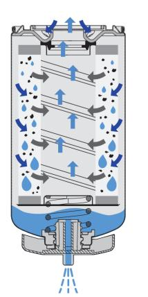
Clean, unfiltered fuel enters the filter through the baffle/thread plate.
