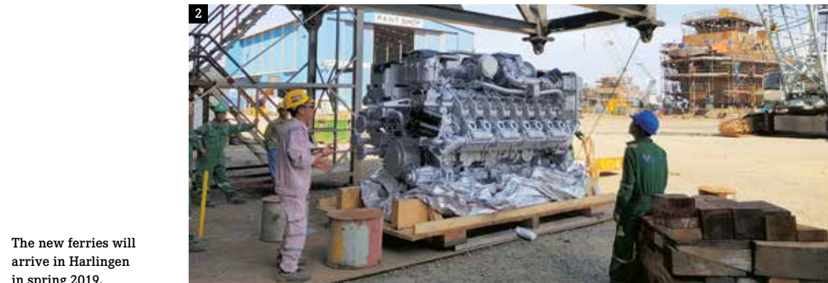
2 At the heart of each ferry are two MTU gas engines with outputs of 1,492 kilowatts each.
