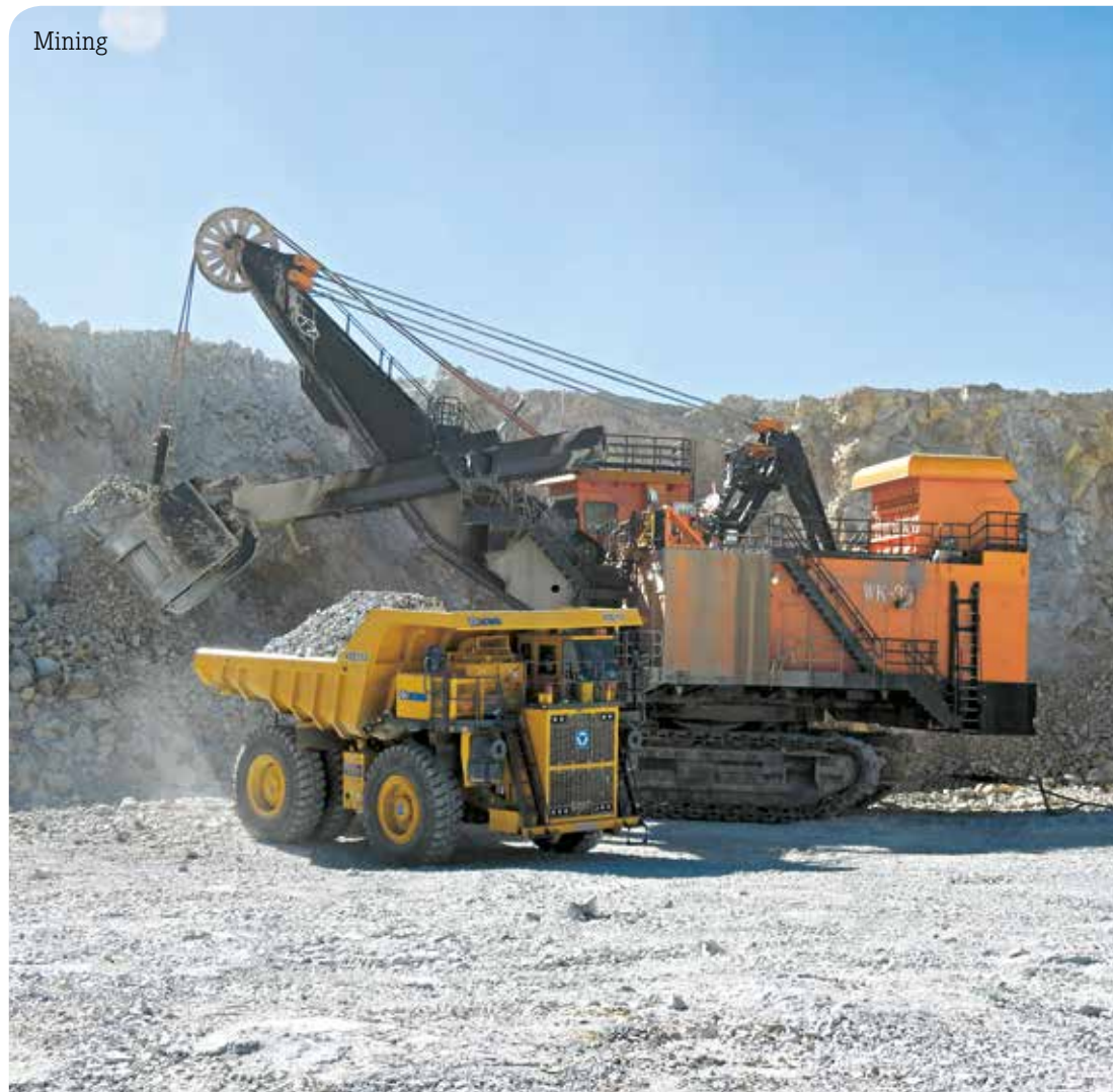
The haul trucks made by Chinese construction machinery manufacturer XCMG can accept payloads weighing up to 110 metric tons.
