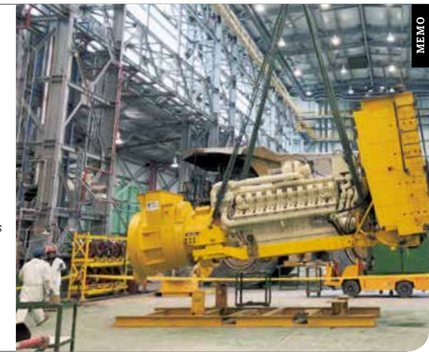
Komatsu haul trucks were retro-fitted with MTU engines at the Antamina Copper Mine in Peru, which lies at an altitude of 4,500 meters.
