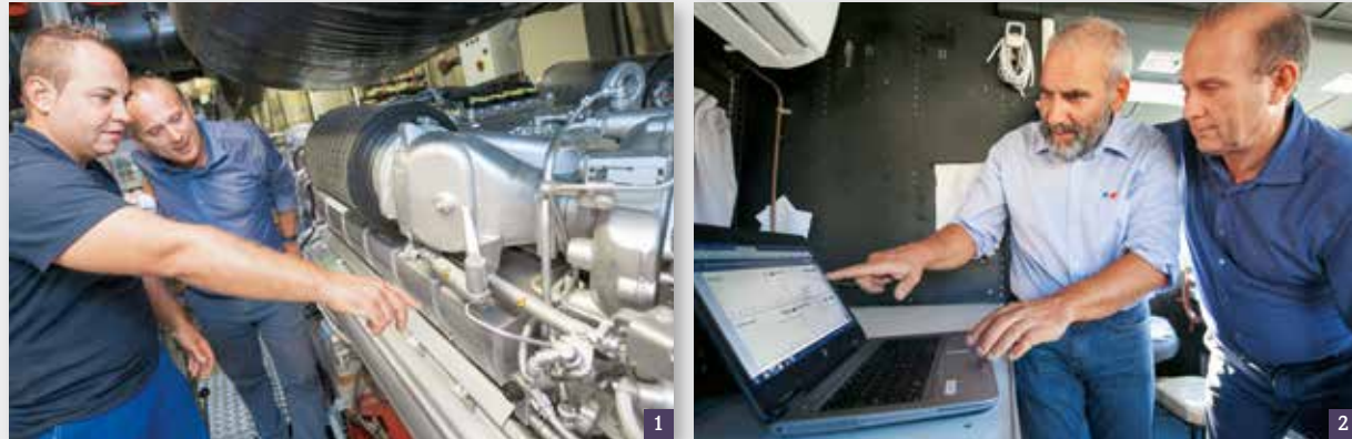
1 MTU Italia Service Technician Matia Lupi (left) supervised installation of the new Series 2000 engines at the beginning of September. The data link was installed as part of the repowering project. “This allows us to respond even to a minor error message and thereby preclude engine failures before they occur,” says Paolo Mazzucchelli, Technical Director of Navigazione Laghi (right). 2 Stefano Gibelli, Technical Manager of MTU Italia (links), showing Paolo Mazzucchelli how he can now use the MTU Go! Manage on his laptop.
