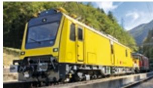
Railroad inspection vehicle
