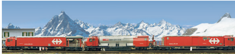
Fire fighting and rescue train
