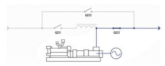
Independent Mode mtu Kinetic PowerPack provides energy as secondary power source, without interruption
