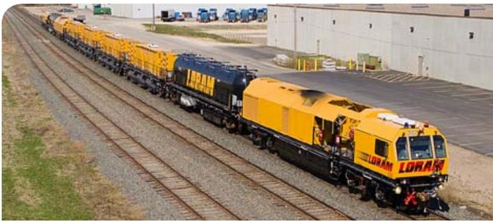
Each grinding car houses four MTU engines: three Series 4000 and one Series 60.
