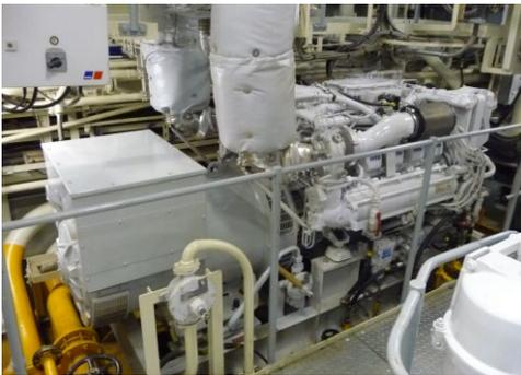
On board the frigates, four gensets based on 8-cylinder Series 2000 engines deliver the power needed to supply all of the electrical consumers.
