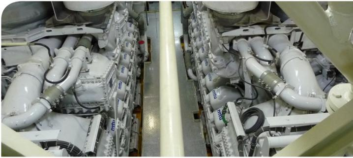
Four 16-cylinder Model 1163 TB 73L engines provide the propulsion needed to take the frigate up to a maximum speed of 27 knots (50 kph). Thanks to their compact design, the new engines fit perfectly into the engine room.
