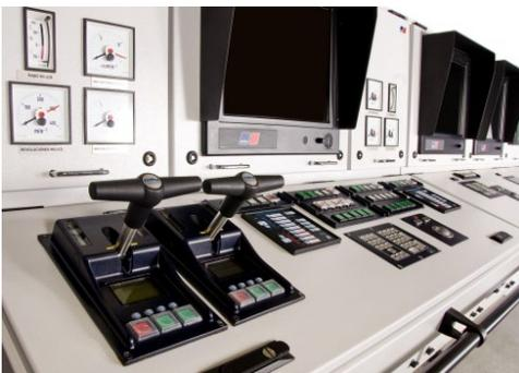
MTU integrated all automation system components for the bridge and engine control room in control panels. After thorough tests, MTU shipped the units to the Colombian shipyard COTECMAR for installation in the frigates.
